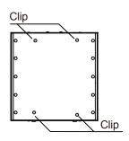
Place charcoal filters to back side of baffle filters. Secure charcoal filters in place by ruber clips. Depending on filter design secure top and bottom of charcoal filters by either rubber clips.
