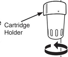
**NOTE:** A newly installed water filter cartridge may cause water to spurt into the icemaker.
