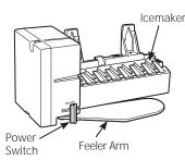
When the refrigerator has been connected to the water supply, set the power switch to ON.
