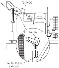
washer on the rod. Reinsert the pin.
