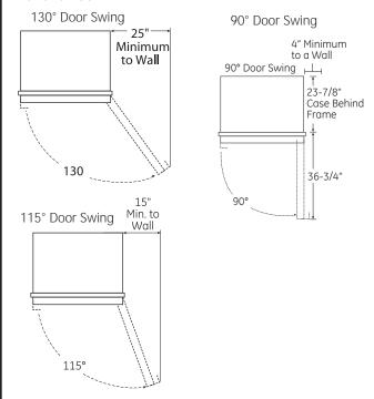
Allow 25" minimum clearance for a full 130° door swing. Allow 15" for pan removal.
