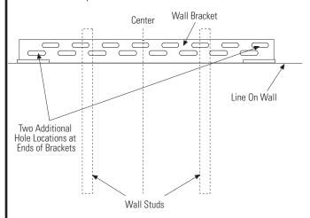
• Mark an additional hole at each end of the bracket. If one of the studs is closer to the end of the bracket, mark an additional hole towards the center of the bracket.
