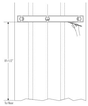
The anti-tip wall bracket has a series of holes. Select 2 holes that match with the located studs. Make sure the holes selected are on the center of the studs. Mark the wall at these points.
