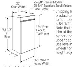
\* Shipping height. The product can be adjusted to fit into a cutout that is 84-1/2" max. height. Note that the top case trim at the front is 1/2" higher and will overlap upper cabinetry or soffit. Use leveling legs and wheels for a maximum 1" height adjustment.
