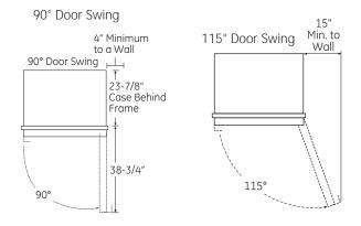
For a 90° door swing, allow 4" minimum clearance to a wall for framed and stainless steel models. If the 90° doorstop position is used, pan access is maintained but pan removal is restricted.
