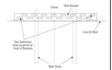
• Mark an additional hole at each end of the bracket. If one of the studs is closer to the end of the bracket, mark an additional hole towards the center of the bracket.
