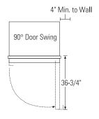
These units are equipped with a 3-position door stop. The factory set 115° door swing can be adjusted to 90° or 130° if clearance to adjacent cabinets or walls is restricted. Order WX14X99 door stop for precise settings between 90° and 130°.
