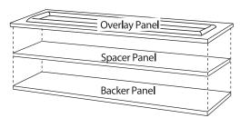
Assemble the overlay panels in the same manner as the door panel.
