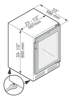
Overall height can be increased by 5/8" (16 mm) by adjusting the feet.
