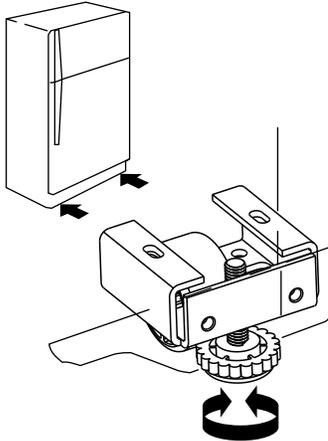
2. Open both doors again to make sure they close as easily as you like. If not, tilt the refrigerator slightly more to the rear by turning both leveling legs to the left; it may take several more turns.
