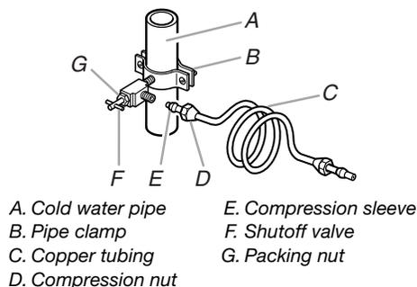
6. Fasten the shutoff valve to the cold water pipe with the pipe clamp. Be sure the outlet end is solidly in the ¼" drilled hole in the water pipe and that the washer is under the pipe clamp. Tighten the packing nut. Tighten the pipe clamp screws slowly and evenly so washer makes a watertight seal. Do not overtighten.
