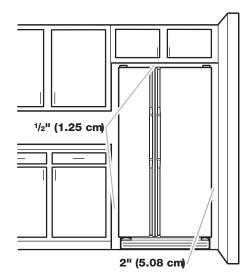
To ensure proper ventilation for your refrigerator, allow for 1/2" (1.25 cm) of space on each side and at the top. Allow for 1" (2.54 cm) of space behind the refrigerator. If your refrigerator has an ice maker, allow extra space at the back for the water line connections. When installing your refrigerator next to a fixed wall, leave a 2" (5.08 cm) minimum space on each side (depending on your model) to allow the doors to swing open.
