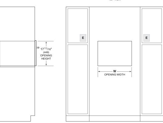
NOTE: 24" (610) and 30" (762) models require the same opening dimensions. Electrical supply must be located in adjacent cabinet within 3' (.9 m) of opening.
