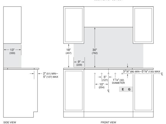
NOTE: Shaded area above countertop indicates minimum clearance to combustible surfaces, combustible materials cannot be located within this area. Maximum facade thickness 1" (25).
