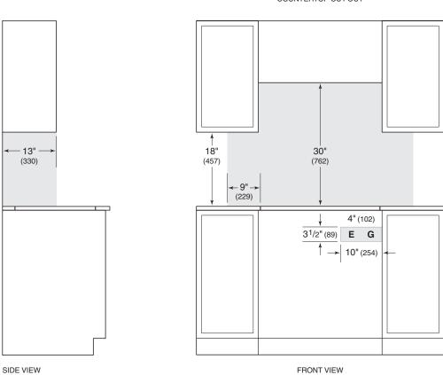
NOTE: Shaded area above countertop indicates minimum clearance to combustible surfaces, combustible materials cannot be located within this area.
