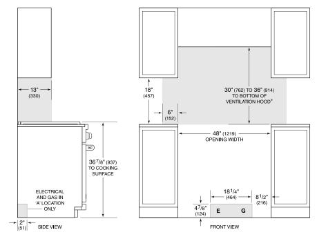
\*Without ventilation hood, 36" (914) minimum clearance countertop to combustible materials, 44" (1118) for charbroiler. NOTE: Shaded area above countertop indicates minimum clearance to combustible surfaces,
