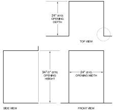
NOTE: 3<sup>1</sup>/2" (89) finished returns will be visible and should be finished to match cabinetry.
