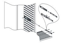
• To remove the shelves out of the rail pull each shelf approximately 3/4 out. Use a long flat screwdriver to press down the right plastic notch as shown in Figure A and at the same time lift the left plastic notch as shown in Figure B. Then proceed to pull out the shelf slowly. Contact our service department if assistance is needed.
