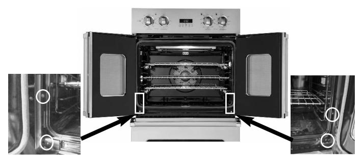
Using a 5/32" allen wrench, adjust screw on each door shown below moving the door that is too high downward and the door that is low upward. You want to adjust both in opposite directions, not just one door. Note that this moves the lower hinge assembly when adjusted.
