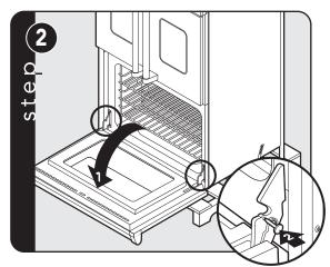
Open lower door completely. Place pin in pin hole. **DO NOT** remove the top/single oven French Doors.
