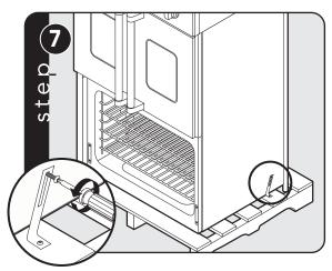
Unscrew pallet screws from side of oven.
