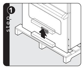
Remove wooden brace on front of pallet.
