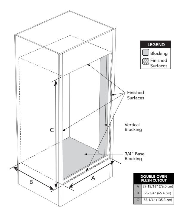
**Note:** To install the professional custom oven in a flush mount application the flush mount accessory kit is required.
