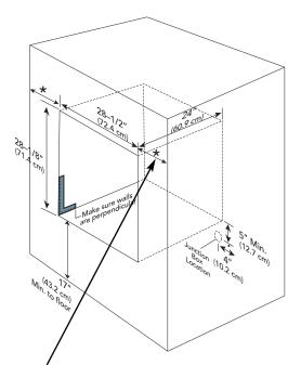
\*French Door Models (VSOF730/CVSOF730) must have a minimum of 18" (45.7 cm) clearance on both sides to allow for door swing
