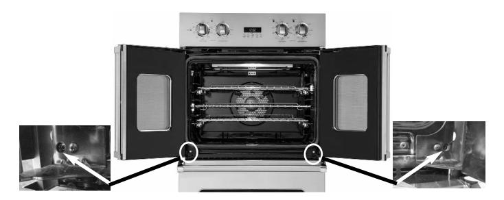
Close doors and check alignment, when alignment is correct, open doors and tighten the lower hinge plate screws that you loosened at beginning of procedure.
