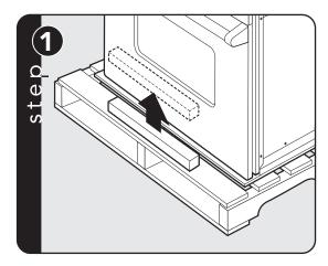
Remove wooden brace on front of pallet.
