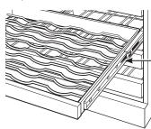
Tab (push tab down on right drawer guide, pull tab up on left drawer guide) When the light pad is pressed and the word ON is displayed, the light will remain on for one hour before automatically turning off. When the light pad is pressed and the word OFF is displayed, the light will come on only when the door is opened.
