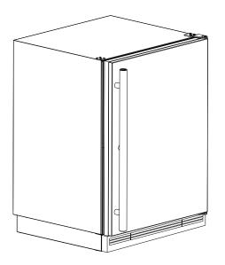
2. Place shell accessory over front and back of cabinet base, aligning holes of shell accessory with the holes on the base. Insert sheet metal screw in back of base.
