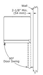
Units have a zero clearance for the door to open 90°, when installed adjacent to cabinets.
