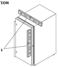
2. If the unit is not level, adjust the legs on the corners of the unit as necessary.
