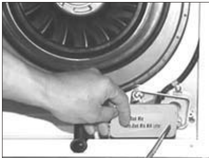
13. Reinstall electrical box cover.
