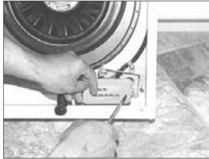
2. Locate electrical connection box inside. Unscrew cover to reveal wiring.
