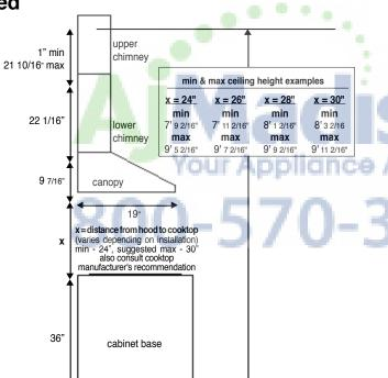
For ducted installations the chimneys are adjustable and designed to meet varying ceiling heights between 7' 9 2/16" and 9' 11 2/16" depending on the distance between the bottom of the hood and the cooktop (distance x in the ducted diagram).
