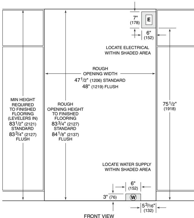
Refer to the full-scale illustrations at the end of this section for specifics on door openings and other specifications.
