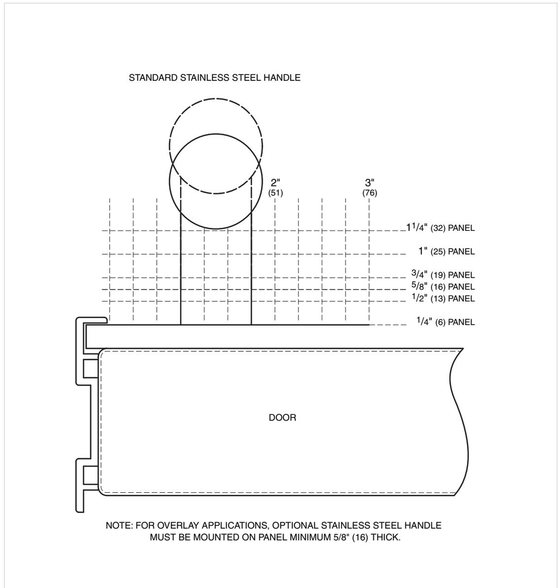
The full-scale illustration above shows handle placement for the standard stainless steel handle on the wrapped stainless steel door and on overlay panel applications shown in the dashed line.
