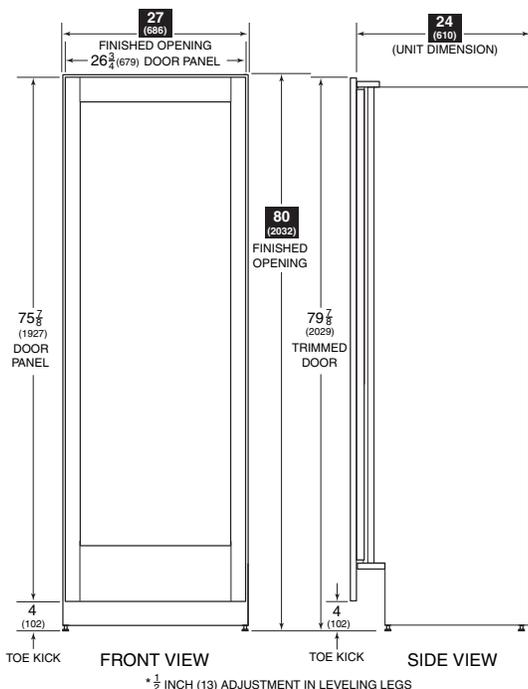
Dimensions in parentheses are in millimeters unless otherwise specified.
