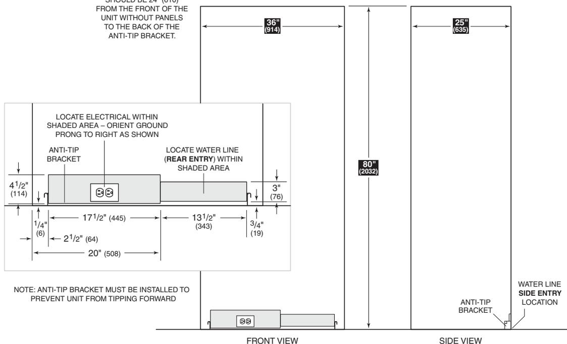
NOTE: ANTI-TIP BRACKET MUST BE INSTALLED TO PREVENT UNIT FROM TIPPING FORWARD
