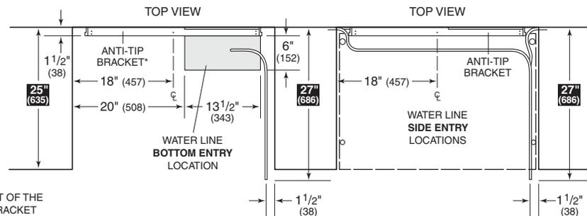
\*PLACEMENT OF THE ANTI-TIP BRACKET SHOULD BE 24" (610) FROM THE FRONT OF THE UNIT WITHOUT PANELS TO THE BACK OF THE ANTI-TIP BRACKET.
