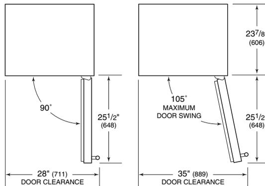
Dimensions in parentheses are in millimeters unless otherwise specified.
