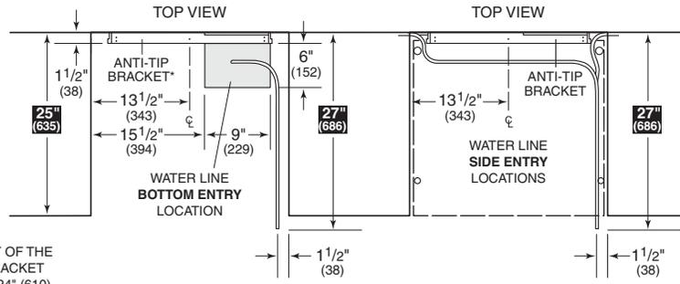
\*PLACEMENT OF THE ANTI-TIP BRACKET SHOULD BE 24" (610) FROM THE FRONT OF THE UNIT WITHOUT PANELS TO THE BACK OF THE ANTI-TIP BRACKET.
