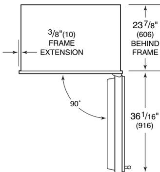
Dimensions in parentheses are in millimeters unless otherwise specified.
