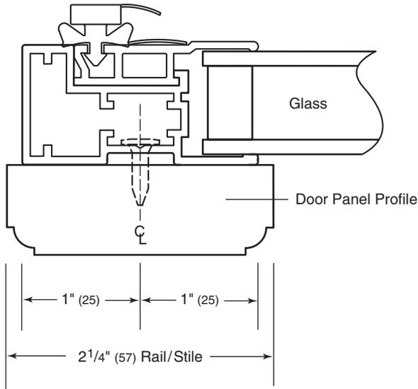
The full-scale illustration shows the door frame profile for Model UC-24B.
