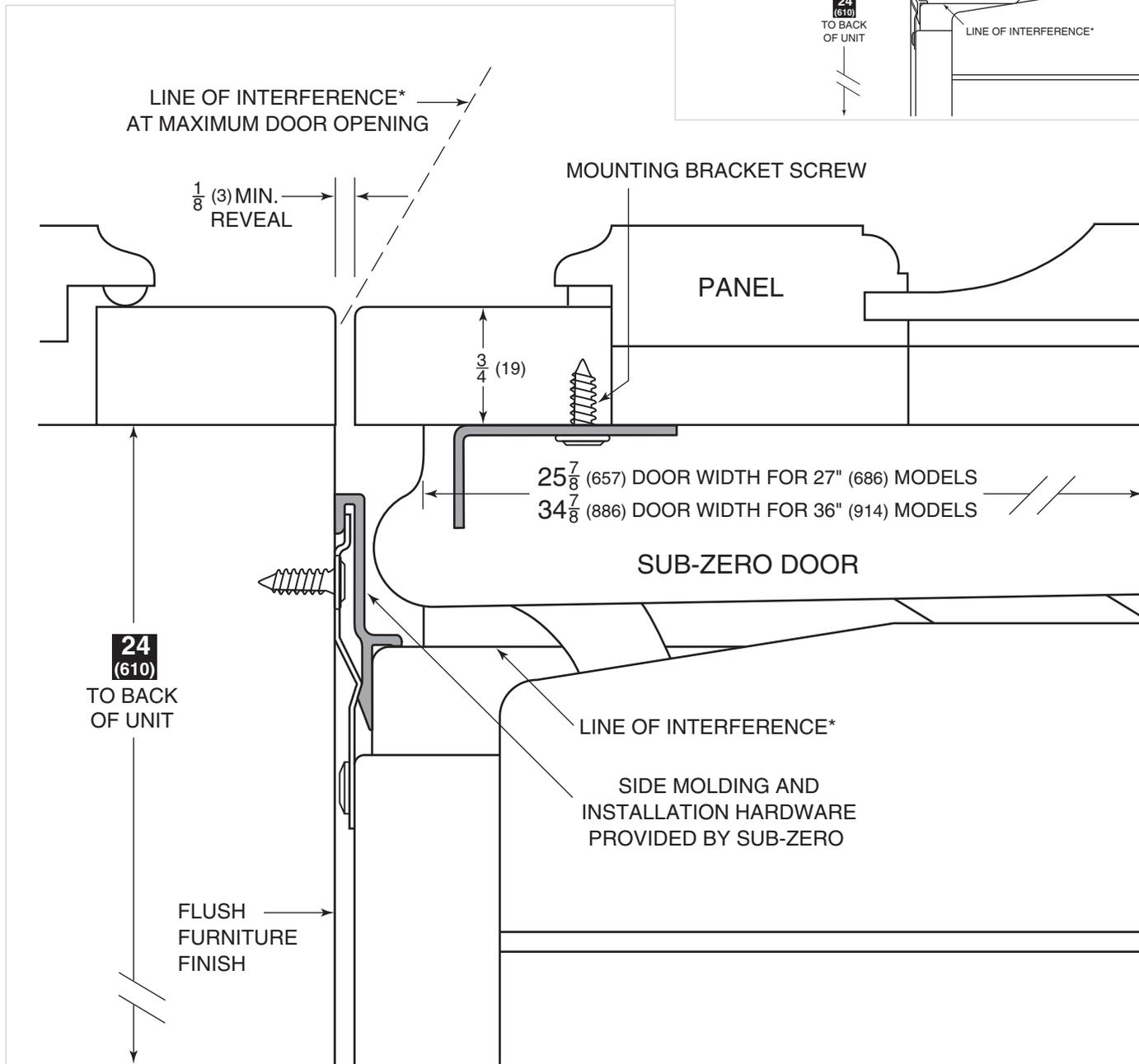
*\*If the panel is thicker than  $\frac{3}{4}$ " (19), it is recommended that you utilize the built-in 90° door stop to prevent damage to the panel and face frame.*
