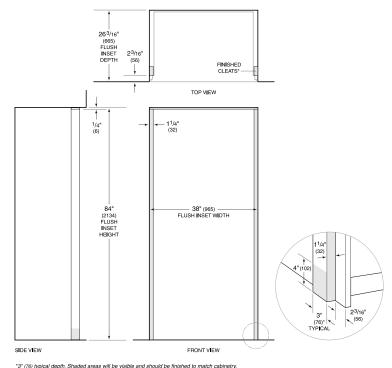
\*3" (76) typical depth. Shaded areas will be visible and should be finished to match cabinetry. NOTE: Shaded line represents profile of unit with <sup>3</sup>/<sub>4</sub>\* (19) panel.
