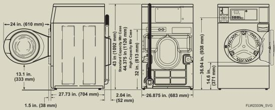
Models Equipped With Drain Hose - Gravity Drain without drain hose
