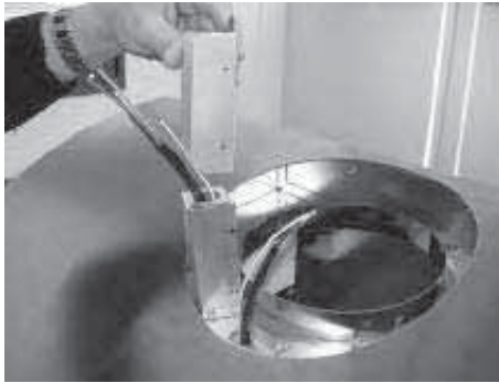
6. Position cover onto external blower wiring box.
