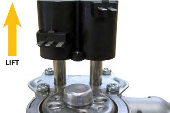
Figure 5 - Lift and remove coil pack.
