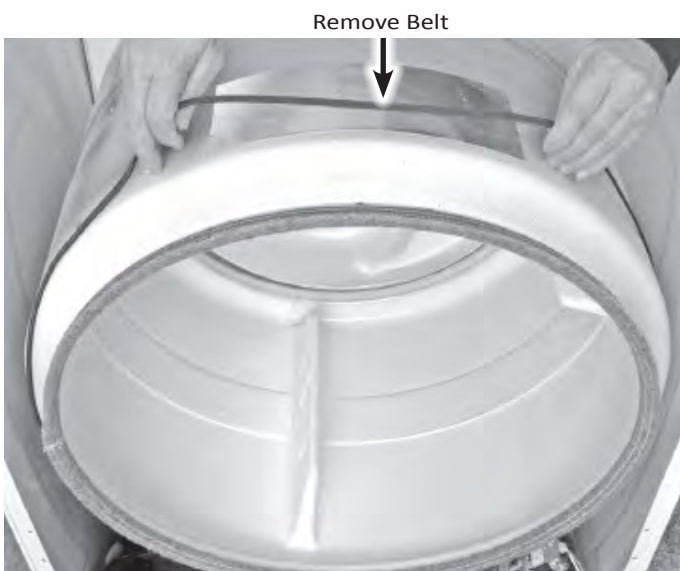
Figure 5 - Remove drum belt.
