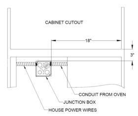
Move the oven with flexible conduit/wires close to the cabinet cutout and feed the wires and conduit through the rectangular cutout located at the rear end of the cabinet cutout base.  Feed the wires in to the junction box and connect the conduit to the junctions box using agency 1/2" conduit connector.
