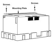
Remove the 2 screws from the mounting plate. This plate will be used as the rear wall template and for mounting.
