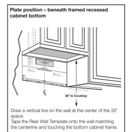
Plate position – beneath recessed bottom
