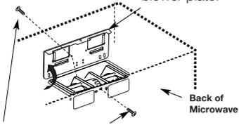
1. Remove and save screw that holds blower plate to microwave.
