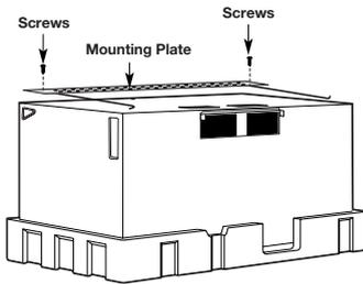
5. Remove the 2 screws from the mounting plate. This plate will be used as the rear wall template and for mounting.
