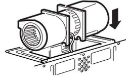
**CAUTION:** Do not pull or stretch the blower unit wiring. Make sure the wires are not pinched.
