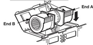
**CAUTION:** Do not pull or stretch the blower unit wiring. Make sure the wires are not pinched.
