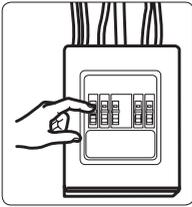
**CAUTION:** For personal safety, remove house fuse or open circuit breaker before beginning installation to avoid severe or fatal shock injury.
