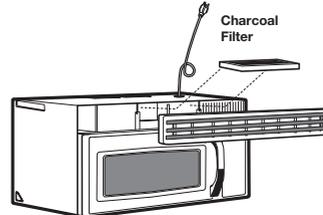
4. Install the charcoal filter. When properly installed, the wire mesh of the filter should be visible from the front.
