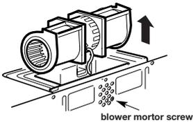
**CAUTION:** Do not touch blade of blower for preventing crack and break. Hold outer case when the blower pull out or back into.
