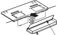
Exhaust Adaptor and Damper is shipped assembled to the filler-upper.
