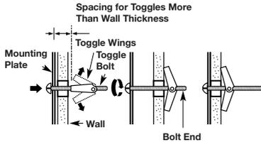
3. Place the mounting plate against the wall and insert the toggle wings into the holes in the wall to mount the plate.
