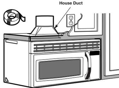
1. Extend the house duct down to connect to the exhaust adaptor.
