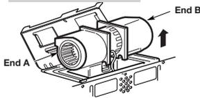
**CAUTION:** Do not touch blade of blower to prevent cracking and breaking. Hold outer case when the blower is removed and re-installed.
