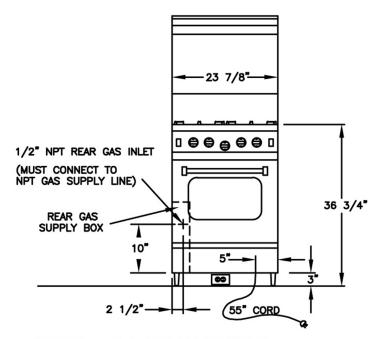
ELECTRICAL CORD LOCATED IN BACK OF UNIT LOCATION OF ELECTRICAL OUTLET MUST NOT BE HIGHER THAN 3" FROM FLOOR IF LOCATED BEHIND THE UNIT OR CAN BE LOCATED IN AN ADJOINING CABINET.
