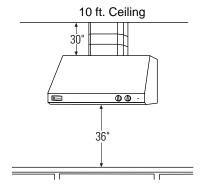
**10 ft. ceilings:** When the hood is installed 36" above the cooking surface, order three 12" and one 6" duct cover accessories.
