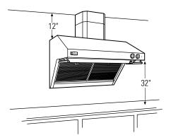
**8 ft. ceilings:** When the hood is installed 32" above the cooking surface and there is no soffit or upper cabinetry, order one 12" and one 6" duct cover accessory.
