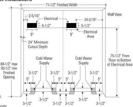
If you are installing two units, side by side, the installation space must be 71-1/2" wide. Additional cutout width may be required when side panels are used. Add side panel thickness to the finished cutout to calculate rough-in width.
