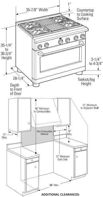
Allow 12" minimum clearance to an adjacent wall on each side.
