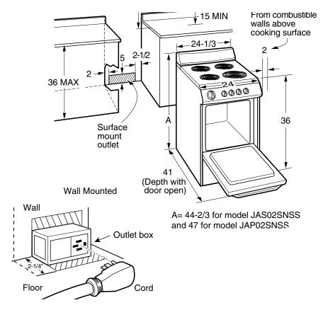
Recommended acceptable electrical outlet area. Orient the electrical receptacle so the length is parallel to the floor.
