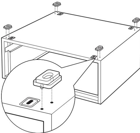
**NOTE:** The support pads should be installed on the dryer only. DO NOT INSTALL THESE PADS ON THE WASHER PEDESTAL.
