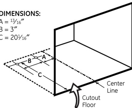
**C** Remove the template and drill two holes for the anti-tip brace.
