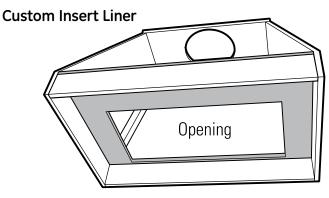
The custom canopy must be sized to fit the insert sleeve. Construct the canopy with an opening that is:  $26\text{"W} \times 13-3/16\text{"D}$
