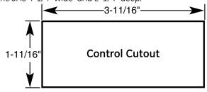
We recommend that the cutout in granite or other hard surfaces be made before the countertop is installed.
