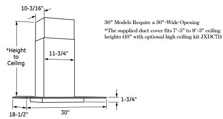
The vent hood must be installed 24" min. and 36" max. above the cooking surface. The hood installation height above the cooking surface depends upon ceiling height. The telescopic duct cover conceals the ductwork running from the top of the hood to the ceiling.
