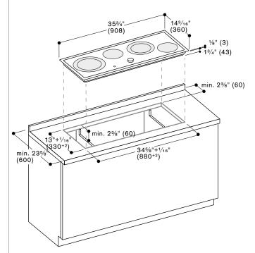
Immersion depth in the area of the electric fitting/conduit is 23/8".
