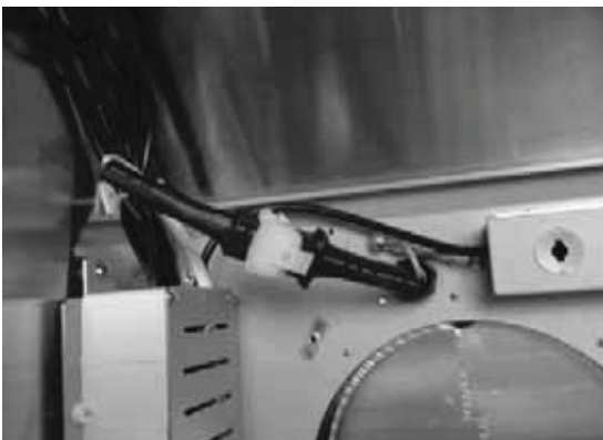
5. Connect 6 pin male connector from remote blower wiring to 6 pin female connector on control board box.
