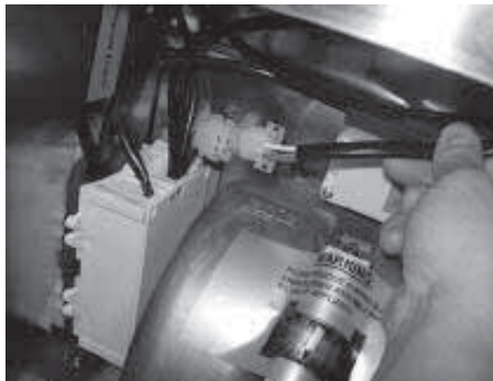
8. Attach long capacitor connector to control board connector.
