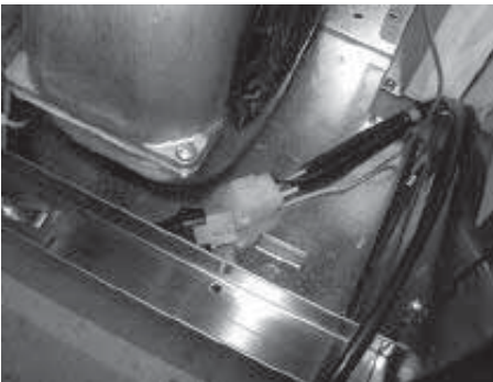
7. Attach short capacitor connector to blower connector.
