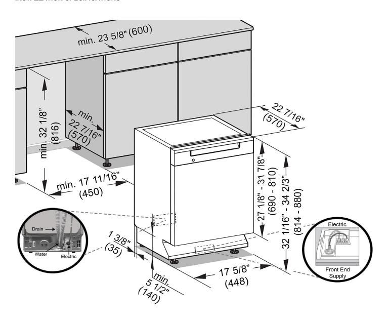
**Drain** - 4 ft 11 in (1.5 m) flexible drain hose.
