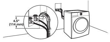
See requirements for floor standpipe drain system.
