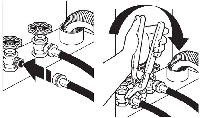
**NOTE:** Do not overtighten, use tape, or sealants on the valve. Damage to the valves can result.
