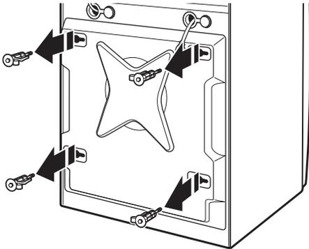
4. Once all 4 bolts are removed, discard the bolts and spacers. Then push the power cord plug into the opening on the right side of the rear panel and pull the power cord through the opening on the left side of the rear panel and close holes with the attached cap. Do not pull plug end of power cord through the right side hole.
