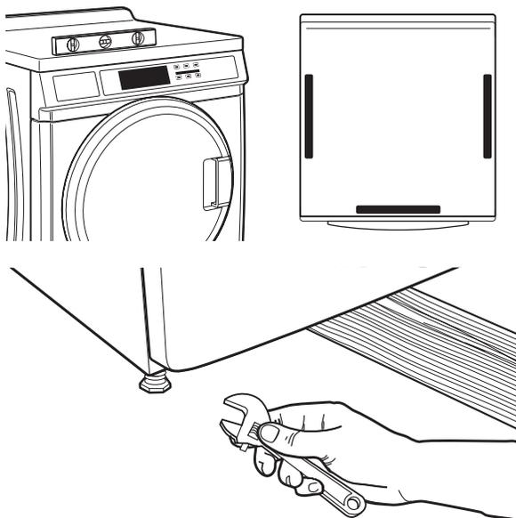
If the washer is against a wall, move the washer out slightly before tipping back. If the washer is not level, first prop the front with a wood block and adjust the feet as necessary; then, prop the back and adjust feet as necessary. Repeat this step until washer is level.
