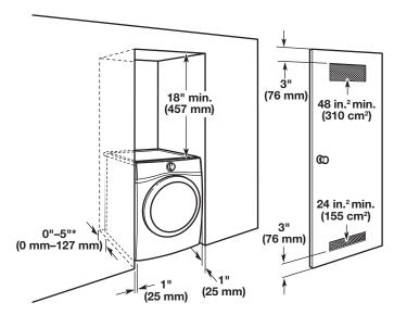
\*0" (0 mm) spacing is allowed for straight-back venting only. For steam models only, inlet hose must not be kinked.
