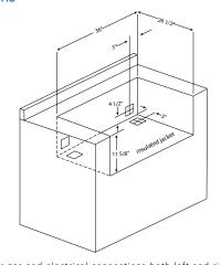
4" square holes for gas and electrical connections both left and right sides(rear or bottom access). Make these holes in the frame based on your requirements. 120V GFI outlet must be located within 6' of the 4" hole.
