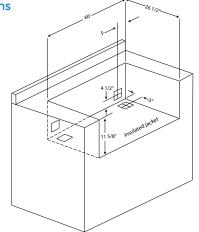
4" square holes for gas and electrical connections both left and right sides(rear or bottom access). Make these holes in the frame based on your requirements. 120V GFI outlet must be located within 6' of the 4" hole.
