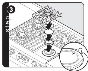
Burner heads and bases are packed in cardboard top pack with the grates. Place burner bases on top of the burner flanges and burner heads on top of the burner base. Place burner grate on top of grate support.
