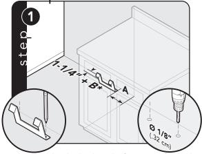
Locate anti-tip bracket hook on the floor Dim A from side cabinet and 1-1/4" (3.2 cm) from rear wall when using an island trim or high shelf. If using an 8" (20.3 cm) backguard, add Dim B to the 1-1/4". Mark and drill 1/8" (.32 cm) holes where bracket will be located.
