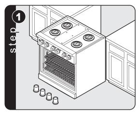
Legs are packed in cardboard top pack. **Note:** Legs should be installed near to where appliance is to be used, as they are not secure for long transit.
