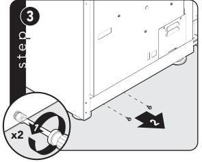
Remove two screws from back of range.
