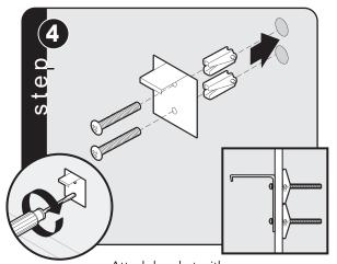
Attach bracket with mounting hardware provided.
