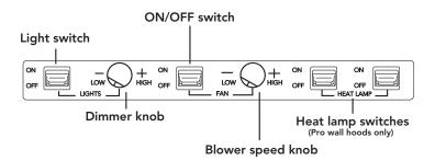
**ON/OFF switch**—Starts and stops the blower. When turned on the blower will operate at the previous setting of the speed control.
