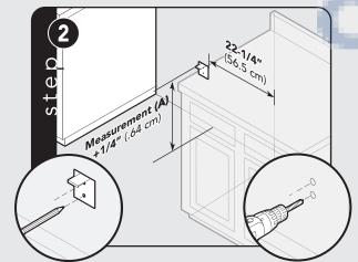
Locate anti-tip bracket on rear wall with the top left corner at measurement (A) plus 1/4" (.64 cm) from the floor and 22-1/4" (56.5 cm) from where the right side of range (facing range) is to be located.
