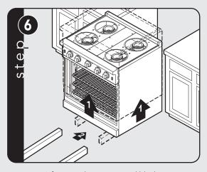
Lift unit and prop on wood blocks.
