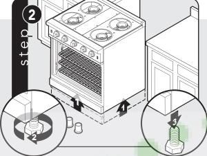
Note: It is strongly recommended that a pallet or lift jack be used rather than tilting. Raise unit about a foot. Unscrew temporary legs from
