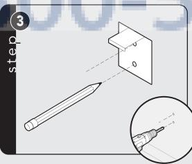
Mark and drill holes where bracket will be located
