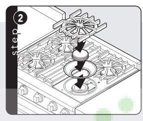
Burner caps and burner bowls are packed in styrofoam top pack with the grates. Place burner bowl in grate support and burner cap on top of burner. Place burner grate over burner cap and on top of grate support.
