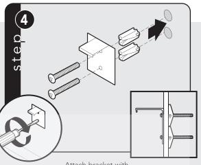
Attach bracket with mounting hardware provided.
