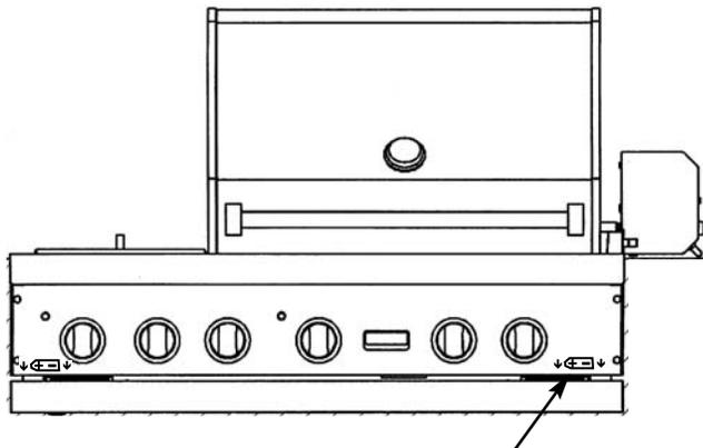
Round black cap which holds battery is located underneath control panel and behind drip tray
