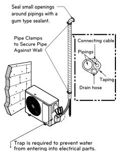
Figure 35: IDU Below ODU - Piping and Trap
