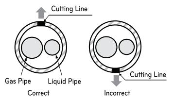
Figure 48: Wrapping Connection Pipe to Indoor Unit's Pipe
