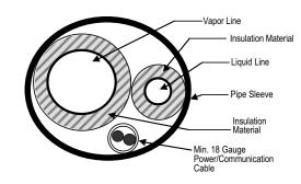
Figure 33: Bundling and Taping
