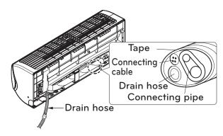
Figure 49: Bundling Pipe and Drain Hose, Rear of IDU
