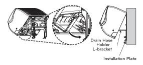
Figure 16: Mounting Bottom of Unit to Installation Plate
