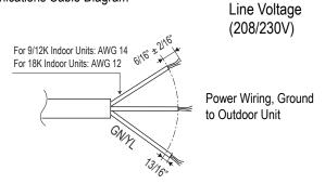
Power Wiring, Ground, Communication Cable From Outdoor Unit To Indoor Unit
