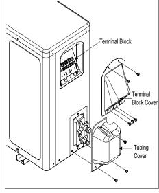
Figure 42: LSU180HSV4 Outdoor Unit Piping Connection.
