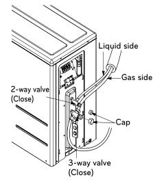
Figure 56: Removing the Service Valve Caps on LSU180HSV4 Outdoor Units
