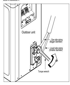
Table 16: Torque Wrench Tightening
