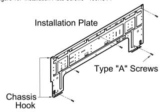
Figure 12: Installation Plate - 180HSV4
