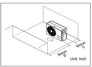
Figure 7: Clearances Where There are Obstacles Above and on Both Air Inlet and Outlet Sides (Obstacle on the Outlet Side is Lower Than the Outdoor Unit)
