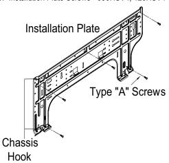
Figure 10: Installation Plate Screws - 180HSV4
