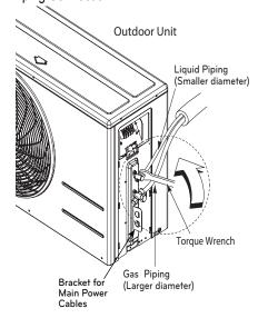
Figure 40: LSU180HSV4 Outdoor Unit Connection Cover Removal.
