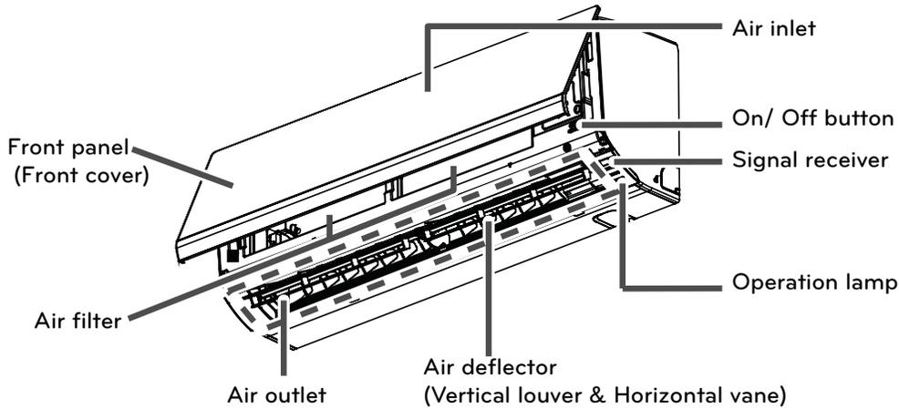
Figure 1: Art Cool Mirror Indoor Unit Basic Components
