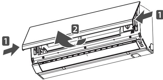
Figure 15: Detaching Filter from Indoor Unit
