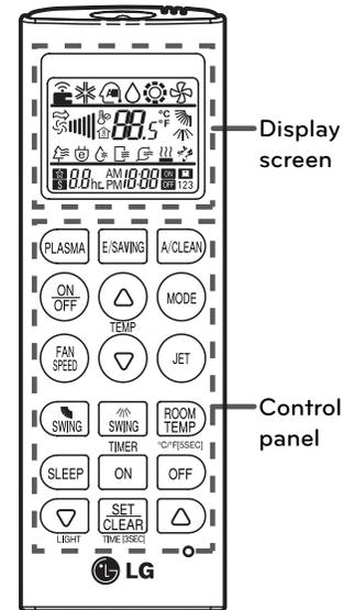
Figure 3: Single Zone Art Cool Mirror Remote Controller - Model AKB73635606
