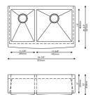
KHF204-33 32 7/8" x 20 3/4" x 10" Min Cabinet Size: 36" Matching Grid: KBG-204-33-1 and KBG-204-33-2 Drain Model #: BST-1 & ST-1
