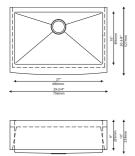
KHF200-30 29 3/4" x 20 3/4" x 10" Min Cabinet Size: 33" Matching Grid: KBG-200-30 Drain Model #: BST-1
