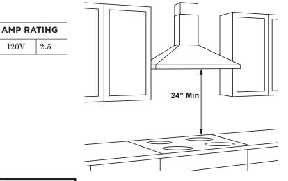
36" Models Require a 36"-Wide Opening \*The supplied duct cover fits 7'-4" to 9'-0" ceiling heights (10' with optional high ceiling kit JXDC72) 9-7/8" 18-1/2" 36"
